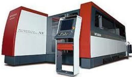
Maquina corte a laser NX3015, 4500 watts.
